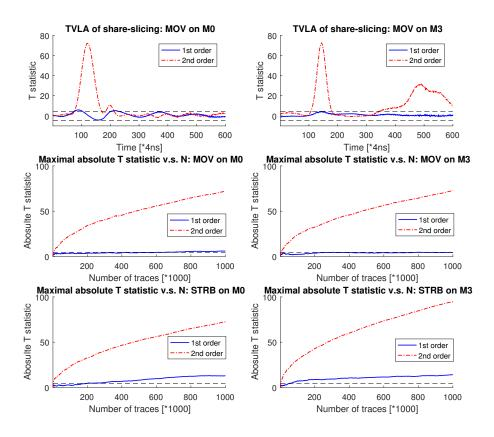
Figure 5: Instruction-wise leakage analysis: MOV/STRB
