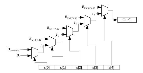
**Figure 2:** Logic function for a single output bit of a 32-bit wide barrel shifter, as found in the ARM ALU. An input word B, is rotated by an amount s to produce a result Out. Note the intermediate nets  $I_x$  at each stage of the circuit.
